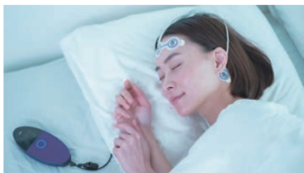
InSomnograf, a device to measure brain waves during sleep at home (S'UIMIN Inc., a start-up company from the University of Tsukuba)
